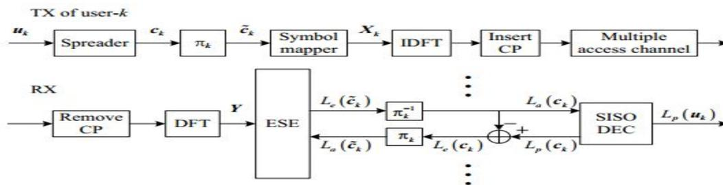
Fig. 1. Transmitter of user- $k$  and receiver in the uplink of an OFDM-IDMA system.
