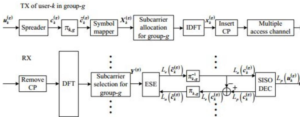
Fig. 2. Transmitter of user-k in group-g and receiver in the uplink of a G-OFDM-IDMA system.
